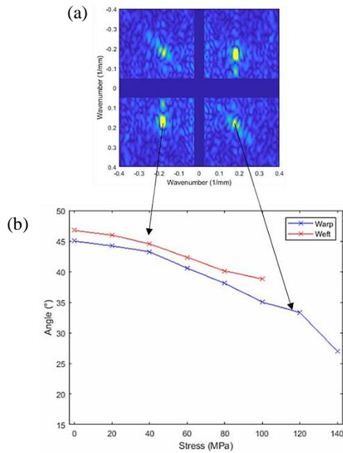
Figure 5: a: Results of the 2DFFT procedure on the sample 1 (no stress applied) with the two tow orientations detected. The two orientations  $+45^\circ$  and  $-45^\circ$  can be obtained. A mirror symmetry due to the 2DFFT is visible. b: Evolution of the two tow orientations with applied stress on sample 1. One of the orientations cannot be measured after 100MPa
