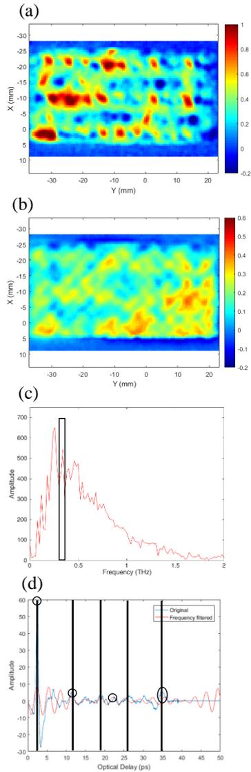
Figure 11: THz C-scan of sample 5 at  $t = 22.67\text{ps}$  (a) before and (b) after applying a 0.3-0.4 THz bandpass filter. (c): Typical THz spectrum at one pixel on sample 5 with the 0.3-0.4 THz frequency band indicated in black. (d): Typical THz signal at one pixel on sample before and after applying the 0.3-0.4 THz bandpass filter.
