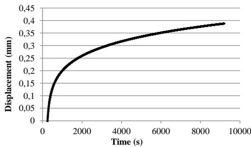
Figure 2: Displacement/time curve from a preliminary creep test performed on a polyamide 6/woven glass fibers with the fiber tows oriented at  $\pm 45^\circ$  loaded at 100 MPa during 9000 s. The curve describes the displacement after 100 MPa is reached.
