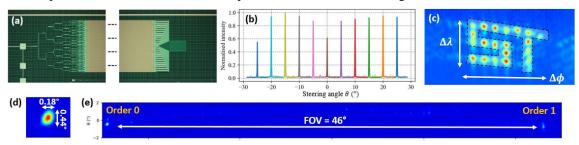
Fig. 2. 256CH OPA characterization (a) Microscope view (x5), (b) OPA field ±25° scanning, (c) Superposition of farfield patterns after a 2D scanning with 100nm wavelength tuning, (d) Farfield pattern on the IR camera, (e) Panorama view of the farfield at -22° deflection angle with side-lobe at 24°.
