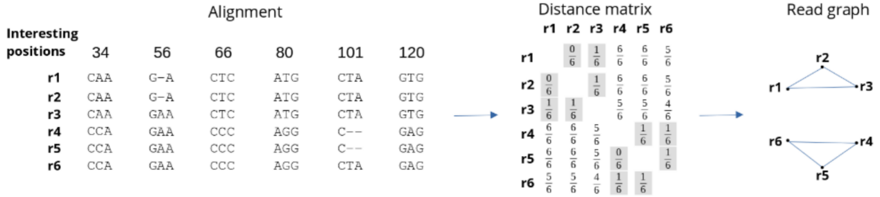
Fig. 5. Generating the read graph from the list of interesting positions with k = 2 . Light gray squares highlight the k closest neighbors of each read in the distance matrix, which become ones in the adjacency matrix of the read graph.
