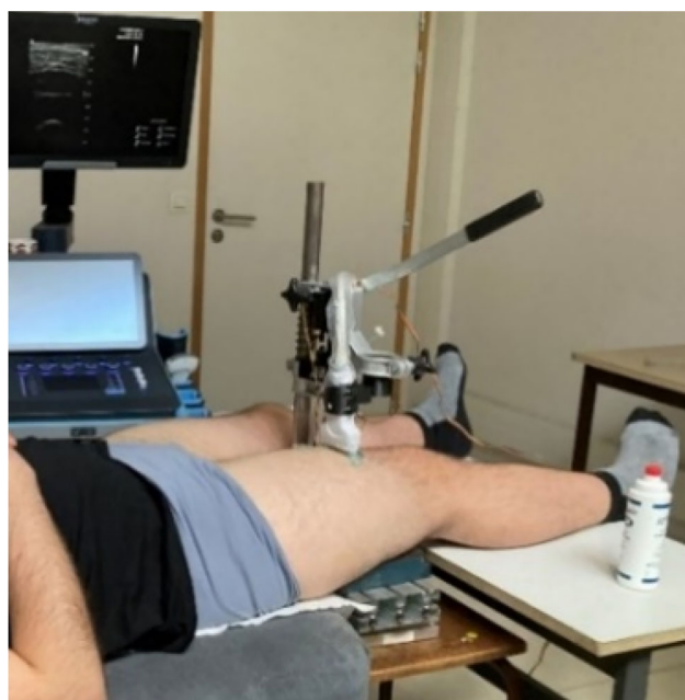
Figure 1. Experimental setup. The ultrasound-based indentation system was placed on a stool positioned in the middle of the right thigh.
