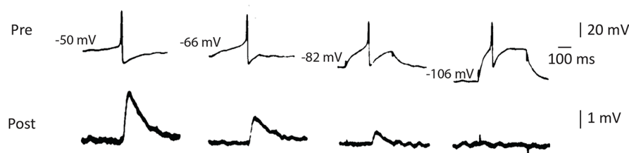
FIGURE 2 | Modulation of AP waveform and synaptic strength by presynaptic membrane potential in invertebrates. (A) Hyperpolarization of the presynaptic element leads to an increase in the spike amplitude and the post-synaptic potential amplitude at squid giant synapse. Adapted with permission from Takeuchi and Takeuchi (1962). (B) Increasing the current applied to emit the spike leads to a decrease in presynaptic spike latency, an increase in spike amplitude and an increased EPSP amplitude at the squid giant synapse. Adapted with permission from Kusano et al. (1967). (C) Depolarization of the presynaptic cell leads to an increase in spike-evoked synaptic transmission at the cholinergic synapse of Aplysia . Adapted with permission from Shapiro et al. (1980).
