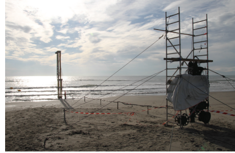
FIGURE 1: Photograph showing the experimental setup and its location on the upper part of Rousty beach. The TLS was fixed on the 4.8-meter high tower standing on the left part of the picture while the scaffold is on the right. The buried sensors can be observed in between.
