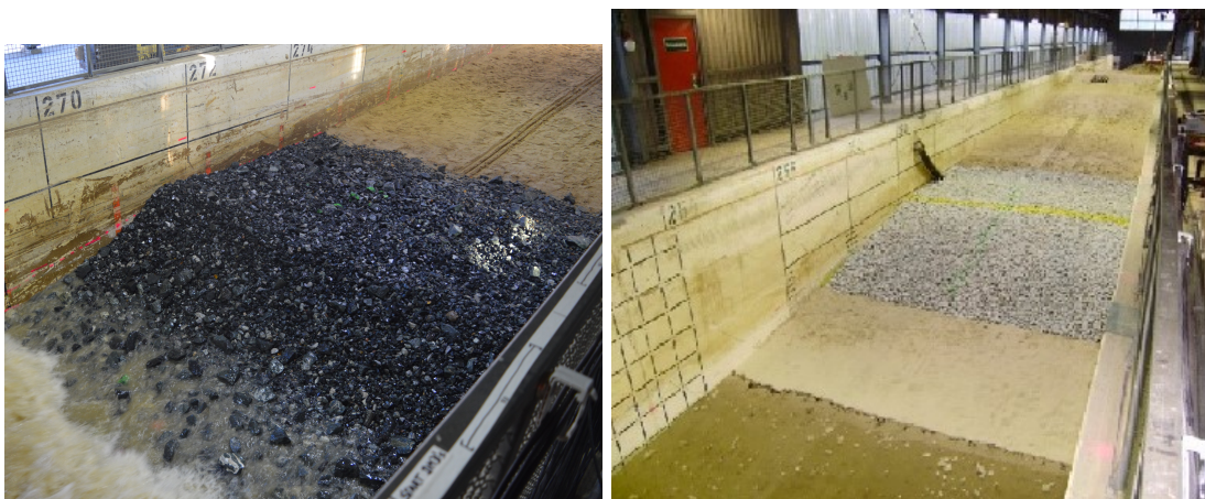
Figure 1: Left) The poorly-sorted revetment. Right) The well-sorted revetment
