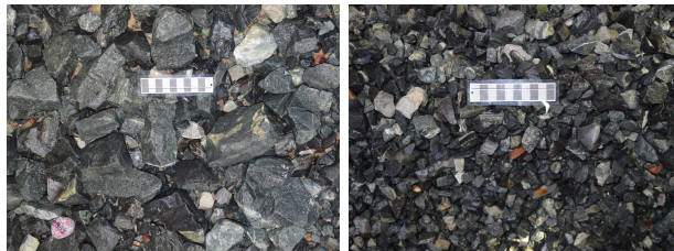
Figure 10: Photo of surface cobbles for the poorly-sorted revetment after standard wave conditions (38 h) at left) the toe of the revetment and right) the crest of the revetment. The total length of the scale bar is 198 mm.
