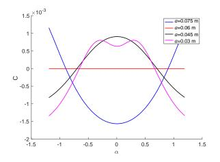
Fig. 4. Influence of the ellipse shape on coactivation range for a E-module.
