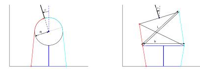
**Fig. 1.** Two possible ways to build a rotating joint actuated by antagonistic tendons: a P-module (left) and a X-module (right)
