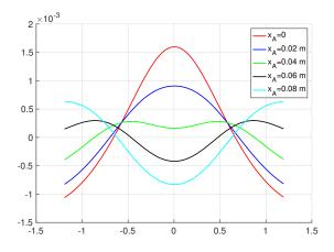
Fig. 5. Influence of the location of tendon base points on coactivation for a E-module.
