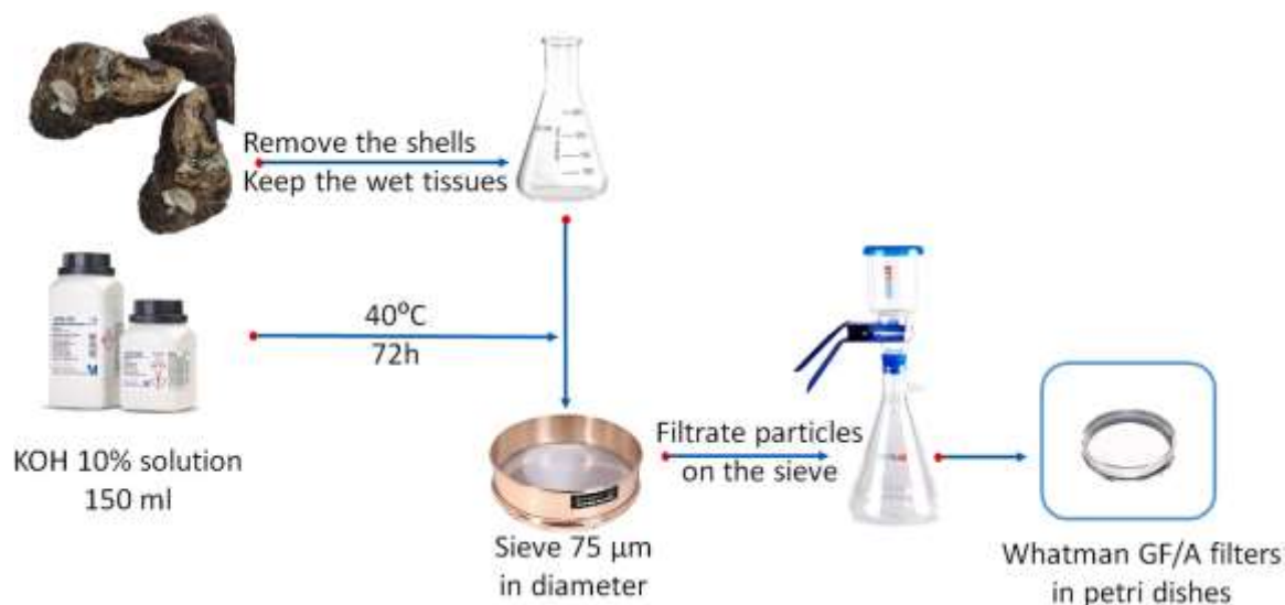
Fig. 2. Protocol for analysis of microplastic (MiP) particles in oyster tissues.
