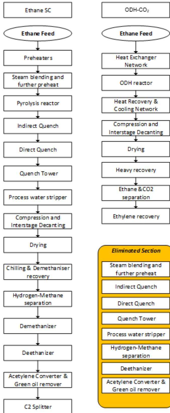
**Fig 9.** Comparison in term of unit operations between SC and OHD-CO<sub>2</sub> ([55])
