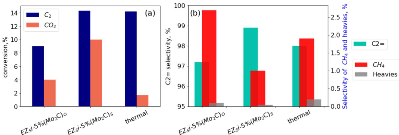
**Fig. 6.** ODH-CO<sub>2</sub> of ethane on EZ<sub>Si</sub>-5%(Mo<sub>2</sub>C)<sub>o</sub>, EZ<sub>Si</sub>-5%(Mo<sub>2</sub>C)<sub>s</sub>, and without catalyst: a) conversion of CO<sub>2</sub> and ethane; b) selectivities to the products (coke-free basis, 700 °C, C<sub>2</sub>H<sub>6</sub>/CO<sub>2</sub>=1/0.74, WHSV = 5.9 h<sup>-1</sup>, average level for 2-5 hours-on-stream).
