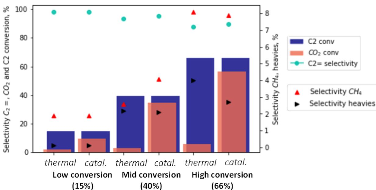
**Fig.8.** Comparison of catalytic (EZ<sub>Si</sub>-5%(Mo<sub>2</sub>C)<sub>S</sub>) and thermal performances in ODH-CO<sub>2</sub> of
