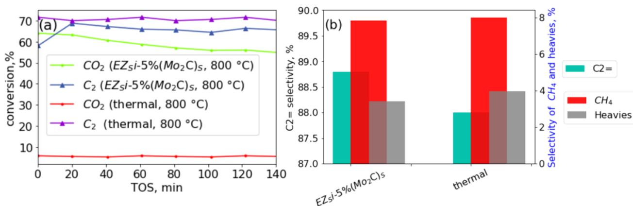
**Fig. 7.** ODH- $\text{CO}_2$  of ethane ( $\text{C}_2$ ) on  $\text{EZ}_{\text{Si}}-5\%(\text{Mo}_2\text{C})_s$  and without catalyst: a) conversion of  $\text{CO}_2$  and ethane as a function on time-on-stream; b) selectivities to the products (coke-free basis,  $T=800^\circ\text{C}$ ,  $P=1\text{ atm}$ ,  $\text{C}_2\text{H}_6/\text{CO}_2=1/0.74$ ,  $\text{WHSV}=5.9\text{ h}^{-1}$ ).
