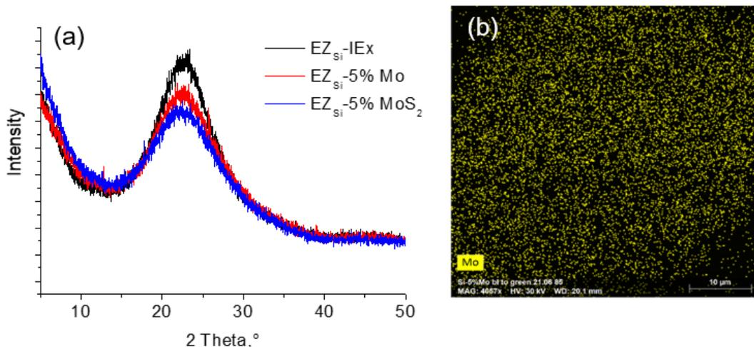
**Fig. 1.** a) XRD patterns of  $EZ_{Si}$ -IEx,  $EZ_{Si}$ -5% Mo,  $EZ_{Si}$ -5% MoS<sub>2</sub>; b) EDX elemental mapping of Mo in  $EZ_{Si}$ -5% Mo.
