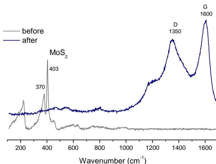
**Fig. 5.** Raman spectrum of embryonic zeolite decorated with sulfide phase before and after the catalytic test at 700 °C over  $\text{EZ}_{\text{Si}}-5\%(\text{Mo}_2\text{C})_{\text{S}}$ .
