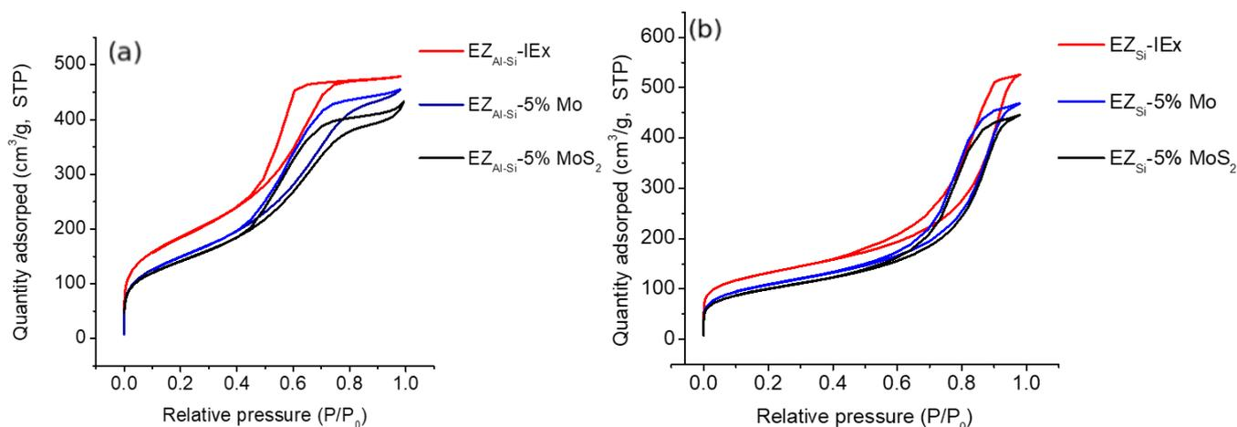
**Fig. 2.** N<sub>2</sub> adsorption-desorption isotherms: a)  $EZ_{Al-Si}$ -based; b)  $EZ_{Si}$ -based.
