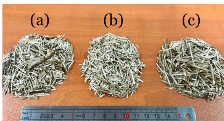
Figure 5. Flax shives: (a) bulk, (b) medium, and (c) large [49].
