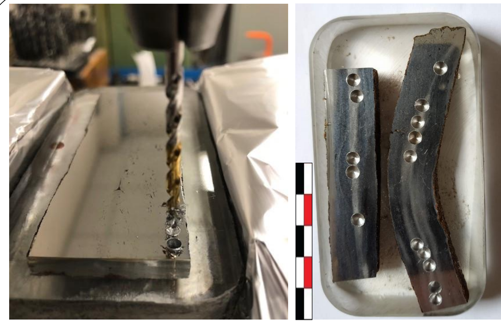
Sampling in the most carburized areas (cementite phase Fe 3 C)
