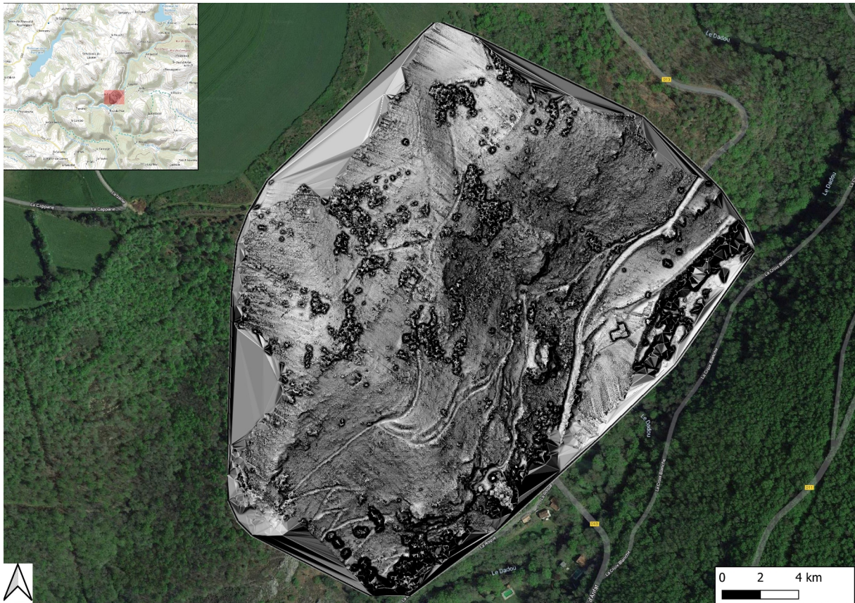
Figure 8 - Terre-de-Bancalié (81), La Roque – mission du 08/03/2022 - Sky View Factor – Rayon 20 px - 16 directions (RVT)
