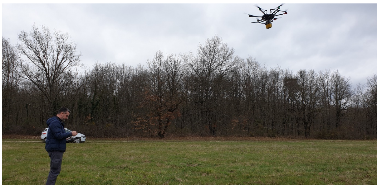
Figure 2-ANR Monumen – mission des 15-17/03/2021 – Survol drone Lidar
