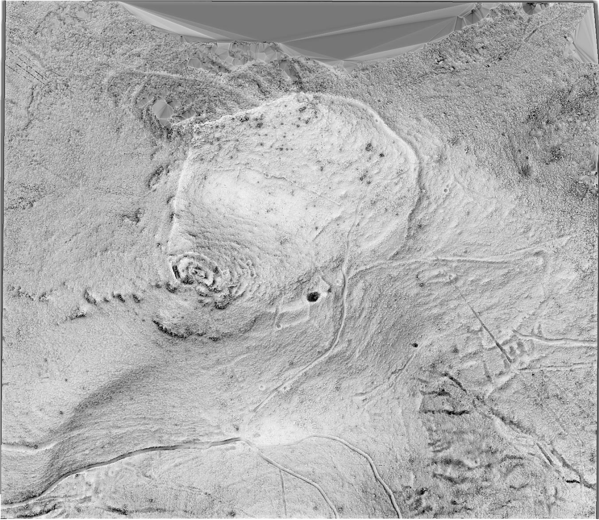
Figure 18 - Ardèche (31) - SVF, Openness Positive et Openness Negative, SVF et Slope à 50% de transparence
