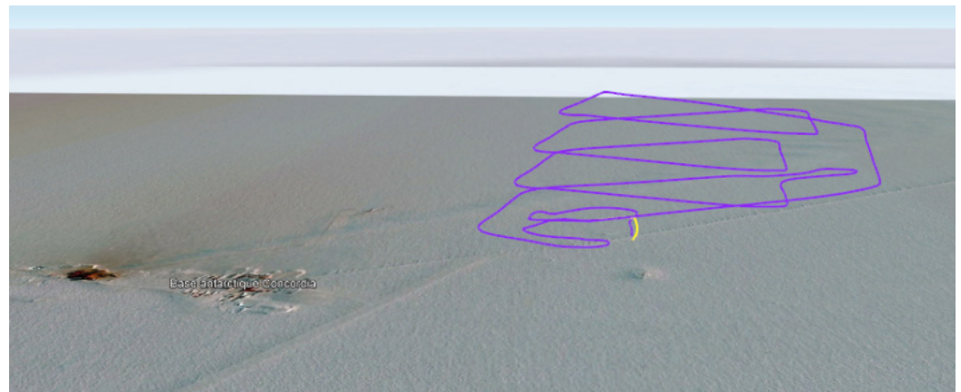
Figure 5. (Top) Hippodrome flight plan (blue line) corresponding to the flight D08 on 2 January 2023 up to 400 m high. The x-axis points towards the East whilst the y-axis points towards the North. In the climbing phase, the N-S runs are performed at a levelled height whilst during the W-E runs the height is increased by 50 m. In the descending phase, the drone flies down on all the straight runs. Note that the blue line is superimposed on the red and green lines. (Bottom) Three-dimensional view of the drone flight (purple line) based on the Keyhole Markup Language (KML) file with the Concordia station at the extreme left. The yellow line represents the ascending part of the vertical take-off phase when the drone is in multirotor mode.
