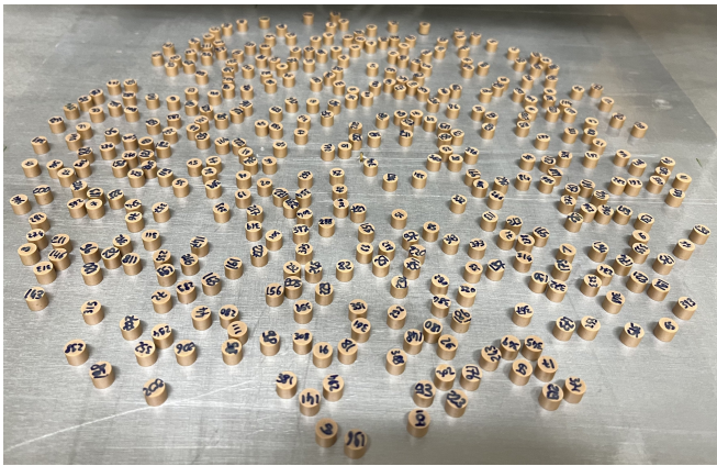
FIG. 8. Image of the 2D disordered array of dielectric cylinders. The top place has been removed to reveal the details of the sample.
