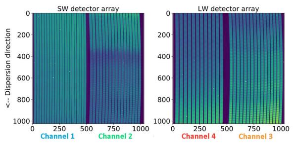
Figure 9. Result of a single exposure on the two detector arrays in the MRS. The illuminated bands correspond to IFU slices. Figure is from Argyriou et al. (2020).
