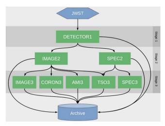
**Figure 14.** Overall flow of the JWST calibration pipeline. Credit: K. Gordon et al. (2023, in preparation).
