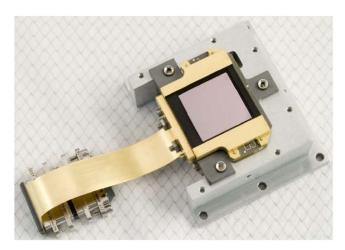
Figure 13. An MIRI focal plane assembly, provided by Raytheon Vision Systems.
