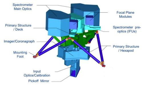
Figure 2. A solid model rendering of the MIRI optomechanical system without its cryocooler. Three mounting feet attach the deck through the hexapod struts to the JWST Integrated Science Instrument Module (ISIM) conductive interface, which is at  $\sim$ 40 K. The MIRI instrument components are suspended off this deck. The entire optics module (OM) shown is surrounded by a radiation shield (not shown). Image credit: P. Samara-Ratna.
