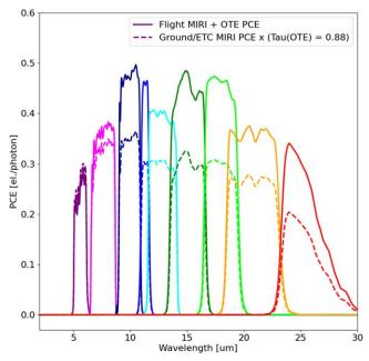
**Figure 15.** The end-to-end photon conversion efficiency of the Webb Optical Telescope Element (OTE) plus MIRI imager filters. On-ground estimates are plotted as dotted lines, where we assume a flat OTE transmission of 0.88. Flight measurements are plotted as solid lines, and are seen to exceed the ground estimates for all filters.
