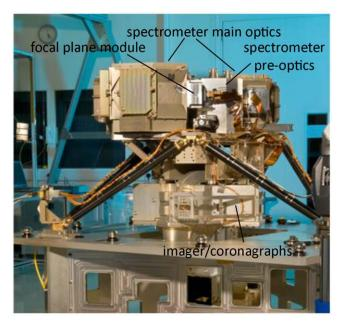
**Figure 3.** The MIRI Flight Model prior to delivery. The OM structure is aluminum; the hexapod truss that mounts it to the telescope is black carbon fiber reinforced plastic. Image credit: STFC/RALSpace.
