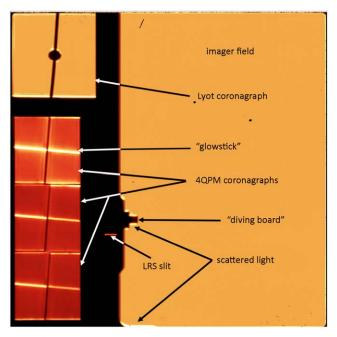
**Figure 4.** Layout of the MIRI imager FOV. The figure also shows the observatory scattered light as seen by the MIRI imager in the F2550W filter, around the "diving board," the bottom rows, and the coronagraphs (e.g., the glowsticks). Image credit: M. García Marín.
