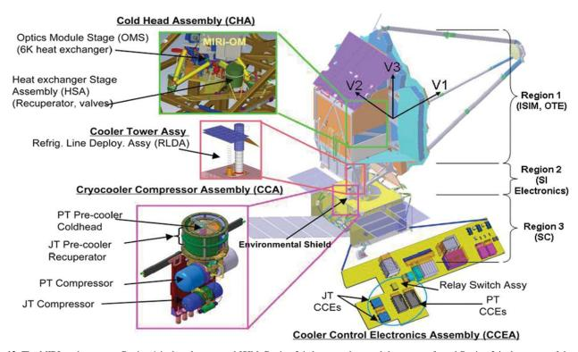
Figure 12. The MIRI cooler system. Region 1 is the telescope and ISIM, Region 2 is between them and the spacecraft, and Region 3 is the spacecraft bus itself.
