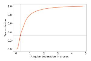
**Fig. A.1.** Transmission of the AGPM coronagraph as a function of the separation, simulated by scanning a point source radially with respect to the center of the coronagraph. The transmission is measured in the central pixel of the point source image and normalized to the unattenuated PSF. The transmission at the expected position of the planet  $\beta$  Pic b, at 0.3", is 32%, identified as a brown dot in the plot.
