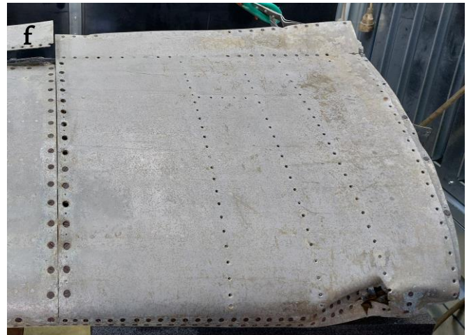
Figure 7. Mechanical cleaning: a) before; b) after treatment; c) consolidation; and chemical cleaning with TAC 5 % w/v applied with Agar gel to 3 % w/v by spray: d) removal of the gel; e) surface before cleaning; f) surface after cleaning.
