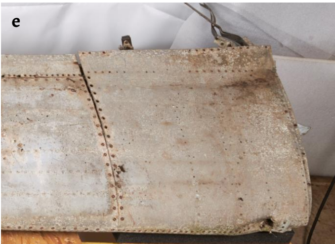
Figure 7. Mechanical cleaning: a) before; b) after treatment; c) consolidation; and chemical cleaning with TAC 5 % w/v applied with Agar gel to 3 % w/v by spray: d) removal of the gel; e) surface before cleaning; f) surface after cleaning.
