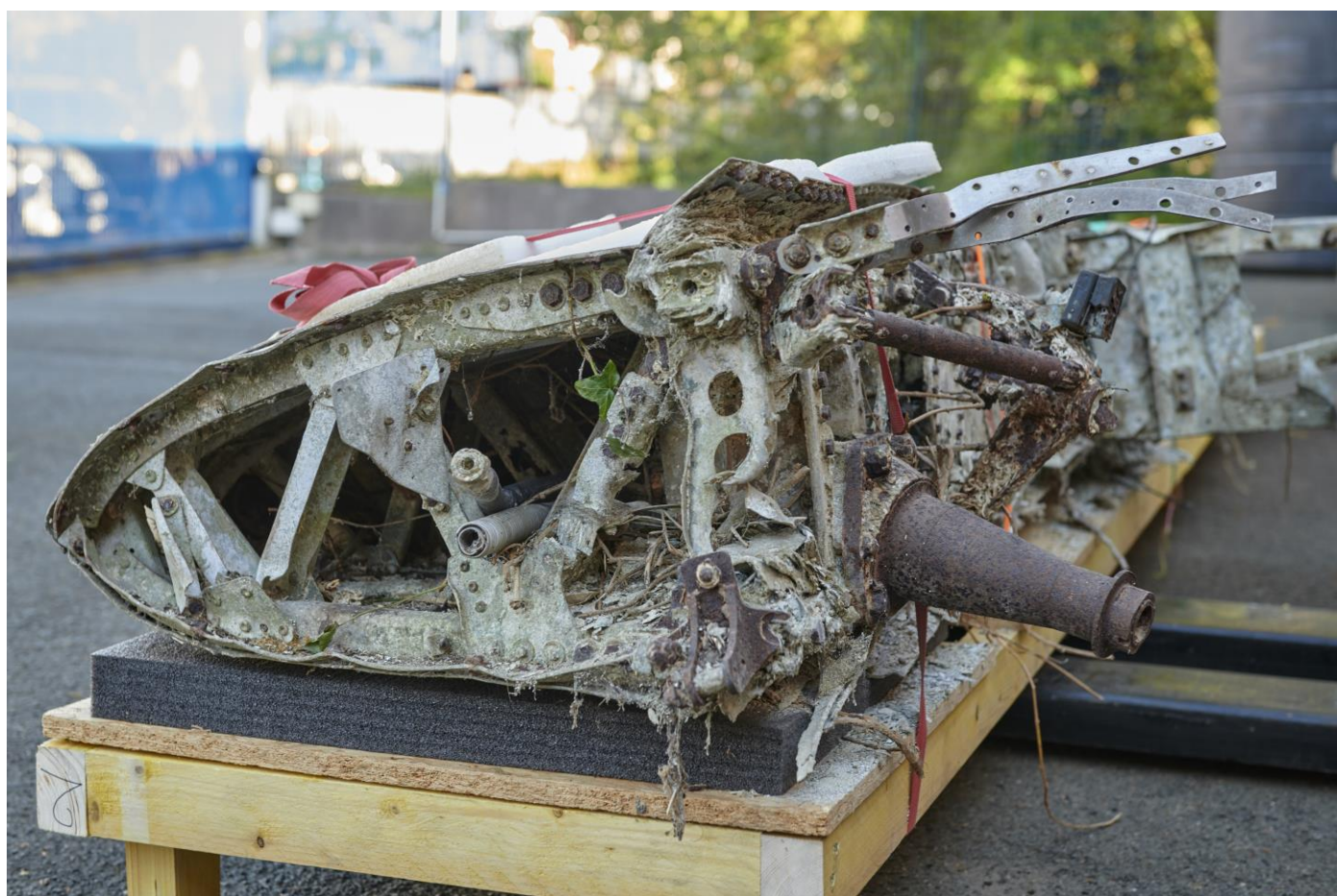
Figure 5. Exfoliation of the spar which caused the Al sheet to buckle.
