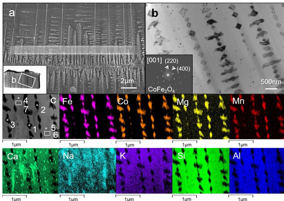
**Fig. 3.** (a) TEM preparation of YL-6 by FIB/SEM with deposition of Pt protection ( $15 \times 1 \mu\text{m}^2$ ) and TEM foil after polishing (lower left); (b) bright-field images of dendrites with the corresponding electron diffraction pattern (lower left); A larger bright-field image (c) and the corresponding elemental maps of dendrites of sample YL-6.
