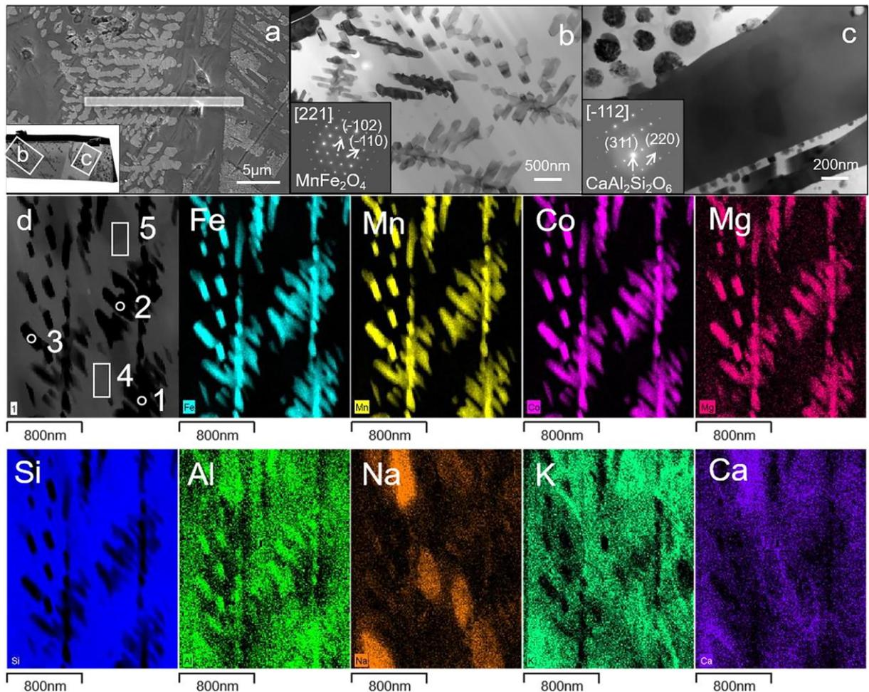
**Fig. 4.** (a) TEM preparation of XD-1 by FIB/SEM with deposition of Pt protection ( $15 \times 1 \mu\text{m}^2$ ) and TEM foil after polishing (Lower Left); (b-c) Bright-field images of L1 and L2 respectively with the corresponding electron diffraction patterns (Lower Left); A larger bright-field image (d) and the corresponding elemental maps of dendrites of sample XD-1.
