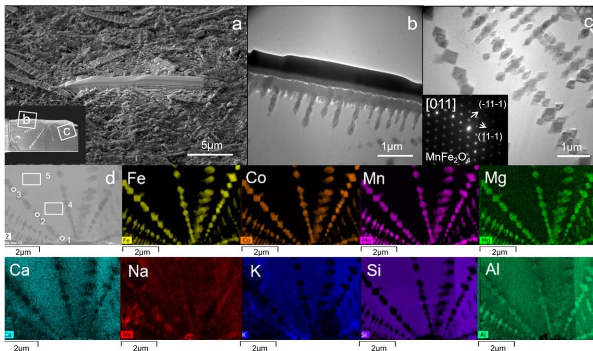
**Fig. 5.** (a) TEM preparation of CH-8 by FIB/SEM with deposition of Pt protection ( $15 \times 1 \mu\text{m}^2$ ) and TEM foil after polishing (lower left); (b-c) Bright field images of dendrites with the corresponding electron diffraction pattern (upper left); A bright field image (d) and the corresponding elemental maps of dendrites of sample CH-8.
