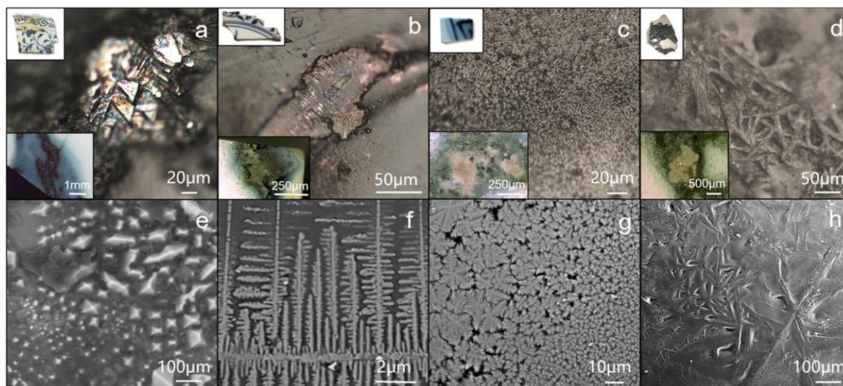
**Fig. 1.** (a-d) Stereomicroscope 3D digital images of 4 typical types of “iron spots” on the glaze surface with corresponding images of samples (upper left) and optical microscope images of “iron spots” (lower left); (e-h) SEM close-up images corresponding to a-d respectively.
