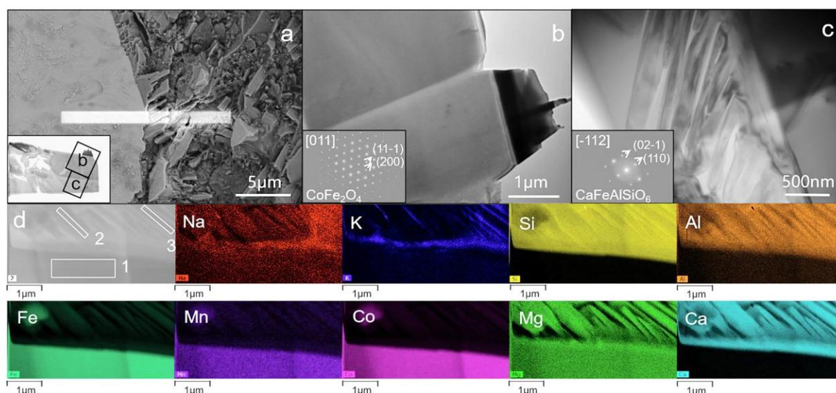
**Fig. 2.** (a) TEM preparation of HW-4 by FIB/SEM with deposition of the Pt protection ( $15 \times 1 \mu\text{m}^2$ ) and TEM foil after polishing (Lower Left); (b-c) Bright-field images of column-like crystals and crystalline block with corresponding electron diffraction pattern (Lower Left); A larger bright-field image (d) and the corresponding elemental maps of crystals of sample HW-4.
