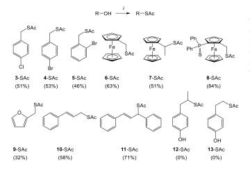
**Scheme 3.** Scope of the thioester (R-SAc) synthesis from alcohols (R-OH) and thioacetic acid; *i*: Conditions- 0.15 molar equivalents of HBF<sub>4</sub> in AcSH, room temperature, 30 min (1 h for **3**, **4** and **5**). Yields were determined on isolated products after extraction and purification by column chromatography.
