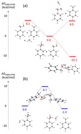
Figure 11. Computed Gibbs energy changes for the interaction between two molecules of benzyl alcohol with (a) one H<sup>+</sup>; (b) two H<sup>+</sup>. The blue and red figures are the Gibbs energies and the black figures are selected bond distances in Å.
