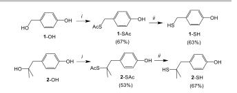
Scheme 2. Synthesis of thiol-phenols 1-SH and 2-SH from the corresponding alcohols 1-OH and 2-OH (isolated yields after purification by column chromatography); *i*: HBF<sub>4</sub> (0.15 mol eq.), AcSH, 30 min; *ii*: NaOMe (2 mol eq.), MeOH, 90 min.
