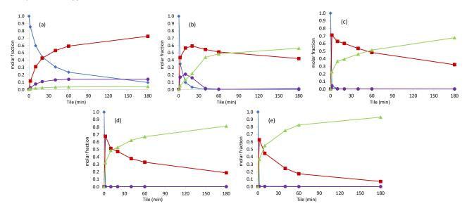
Figure 5. Time evolution of alcohol ( $\blacklozenge$ ), ester ( $\blacksquare$ ), thionoester ( $\blacklozenge$ ) and thioester ( $\blacktriangle$ ) in the reaction of PhCH<sub>2</sub>OH with 0.15 (a), 0.5 (b), 1.0 (c), 1.5 (d) and 2.0 (e) equivalents of HBF<sub>4</sub> per PhCH<sub>2</sub>OH in CH<sub>3</sub>C(O)SH (the PhCH<sub>2</sub>OH/MeCOSH ratio was approximately 0.06 in all samples).
