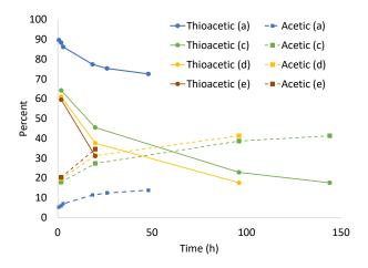
**Figure 7.** Evolutions of the CH<sub>3</sub>COSH and CH<sub>3</sub>COOH fractions with time in the presence of different HBF<sub>4</sub>·OEt<sub>2</sub> amounts. The fractions are derived from integration of the <sup>1</sup>H NMR resonances, with the assumption that the reaction affords equivalent amounts of CH<sub>3</sub>COOH and CH<sub>3</sub>CSSH. The labels (a), (c), (d) and (e) correspond to the conditions used for the experiments shown in Figure 5 (without **14**-OH).
