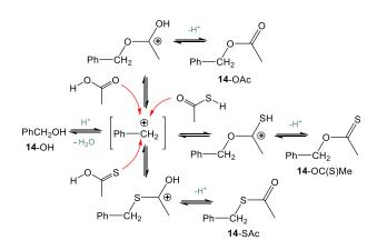
Scheme 4. Proposed mechanism of benzyl alcohol thioesterification.
