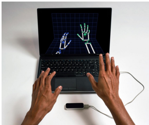
Fig. 4. Example of hands representation by Leap Motion sensor (source: Ultraleap).
