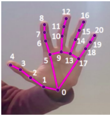
Fig. 3. Points of interest for the hands: real-time detection by MediaPipe engine [20].
