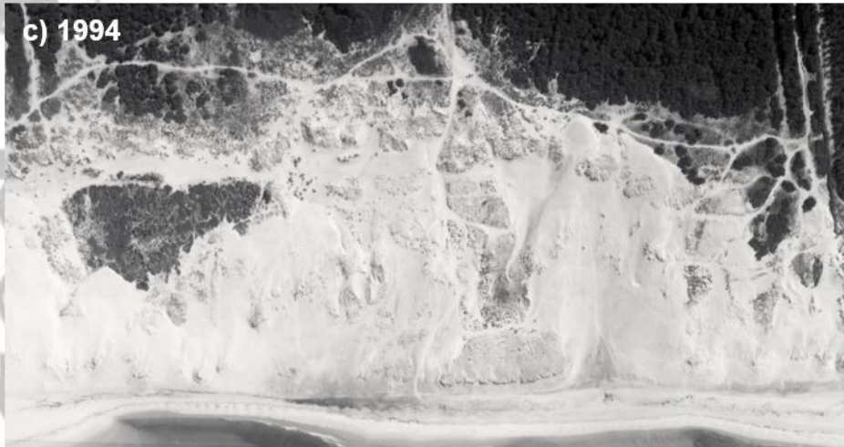
FIGURE 4. Vegetated surfaces on N 5 to N 7 area for (a) 1979 and (b) 2000. (c) Oblique aerial view of the N 5 to N 7 area in 1994 illustrating the destabilization of the system with many blowouts, breaches, large deflation areas and ramps.
