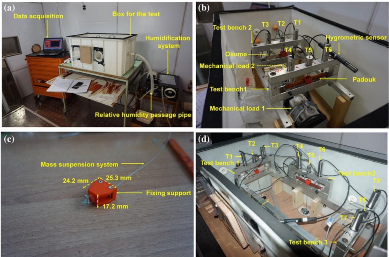
Fig. 2 Experimental setup: **a** overall experimental set-up; **b** view of the two creep benches for the 14-day creep test; **c** plastic support for the application of the load; **d** view of the three creep benches for the 5-day creep test
