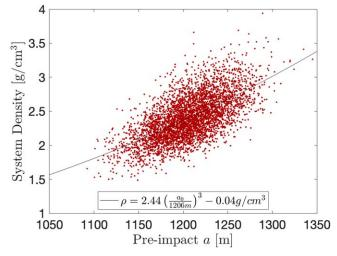
**Figure 9.** System bulk density as a function of the possible pre-impact observable semimajor axis, calculated using a numerical routine considering F2BP dynamics. Accounting for the system uncertainties, including the volumes, the bulk density is  $2.4 \pm 0.3$  g cm<sup>-3</sup> (1 $\sigma$ ), with a dependence on the pre-impact separation.
