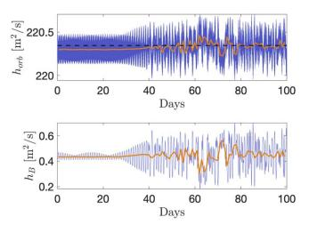
**Figure 17.** The specific orbital angular momentum (top) and secondary angular momentum (bottom) of a system that begins tumbling. As the secondary enters a tumbling state, the orbital angular momentum increases on average. The dashed line corresponds to the nearest equilibrium orbit, and the orange line is a 1 day moving average of the angular momentum. We see an exchange of angular momentum between the orbit and the secondary when the secondary is tumbling.
