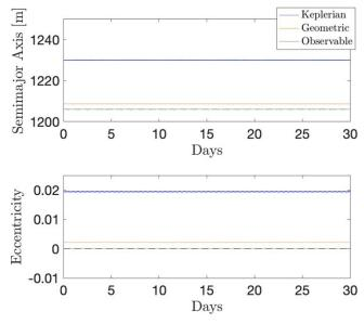
**Figure 1.** Comparison between Keplerian, geometric, and observable elements for an equilibrated binary asteroid, showing the semimajor axis (top) and eccentricity (bottom). The physical parameters are shown as a black dashed line. While geometric elements are an improvement over Keplerian, the observable elements do the best job of describing the physical system.
