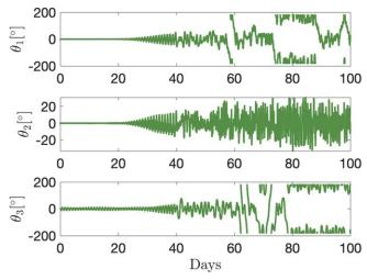
**Figure 16.** The relative 1-2-3 Euler angles (roll-pitch-yaw) of the secondary of an unstable system that begins tumbling. Significant NPA rotation begins at around 40 days into the simulation.
