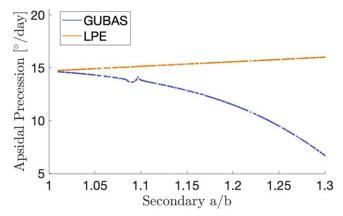
**Figure 24.** The precession rate as a function of the secondary's elongation a/b, calculated using the F2BP dynamics (GUBAS) and the analytical LPEs with the nominal primary  $J_2$ . Including secondary libration in the dynamics results in a decrease in the apsidal precession rate, whereas ignoring it results in an increase. The effect of a resonance is visible near a/b = 1.1, discussed in detail in Agrusa et al. (2021).
