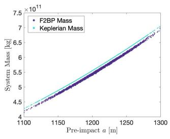
**Figure 7.** System mass calculated using a numerical routine considering F2BP dynamics, along with the system mass calculated using Keplerian dynamics, as functions of the pre-impact observable semimajor axis. Ignoring the F2BP coupling and Didymos oblateness results in a consistently larger mass estimate.
