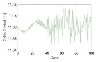
**Figure 20.** Stroboscopic orbit period over time for the tumbling case study in the previous section. Prior to the onset of tumbling, the orbit period experiences small, periodic variations. As the secondary begins to tumble, the amplitude of orbit period variations increases and the periodicity is absent.
