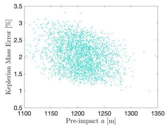
**Figure 8.** Percent error in the calculated mass when ignoring the aspherical shapes and F2BP dynamics, as a function of pre-impact observable semimajor axis. Using Keplerian dynamics results in approximately a 1%–3% error in mass estimate.
