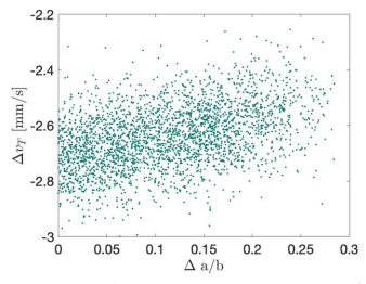
**Figure 22.** Calculated  $\Delta v_T$  as a function of Dimorphos's reshaping of its a/b ratio. For impacts that cause more reshaping, the required  $\Delta v_T$  magnitude to achieve the post-impact orbit period is smaller on average.
