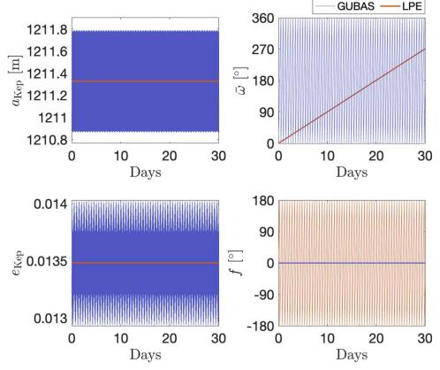
Figure 5. The semimajor axis (top left), eccentricity (bottom left), longitude of periapsis (top right), and true anomaly (bottom right) of a numerical GUBAS simulation compared to the analytical LPE solution for an equilibrated system. The LPE solution shows the true anomaly circulating, while in reality this angle should be zero and the longitude of periapsis should be circulating.
