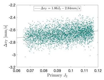
**Figure 11.** Change in along-track velocity as a function of Didymos's possible  $J_2$  gravity coefficient. The magnitude of  $\Delta v_T$  decreases slightly as Didymos's  $J_2$  increases.
