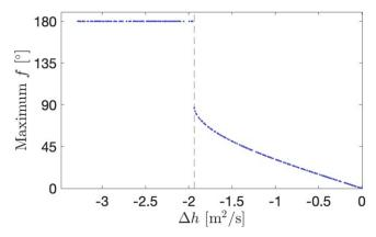
**Figure 2.** The maximum true anomaly as a function of the change in specific orbital angular momentum for an orbit perturbation. There is a discontinuity where the perturbation to the orbit changes the orbital angular momentum enough to push the system out of an equilibrium and the true anomaly switches from librating to circulating.
