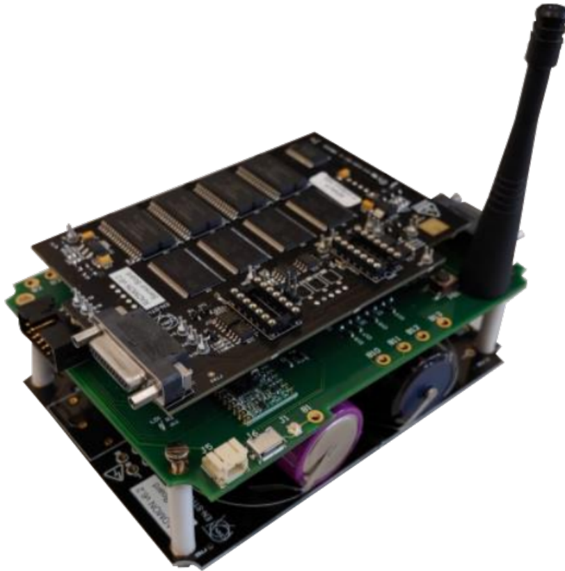
Fig. 3. Battery-powered radiation Monitoring (BatMon) system, a radiation tolerant wireless Internet of Things (IoT) platform for on-field sensor data acquisition [22].
