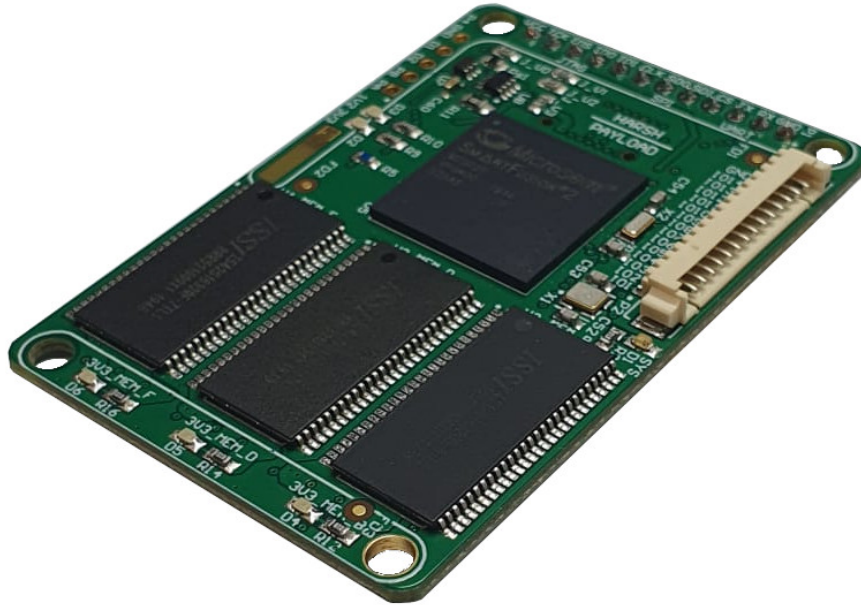
Fig. 5. Harsh Environment CubeSat Payload (HARSH) board [29].
