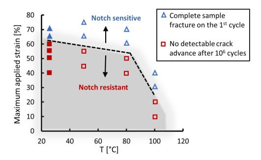
**Figure 3:** Map indicating conditions of applied strain and temperature where either no detectable crack propagation was observed (grey area) or failure was observed in one cycle (white area) for the low Mw sample. The dashed line is a guide to the eye showing the transition between the behaviors. Data points where SIC of the SB is expected to occur are denoted with filled symbols.
