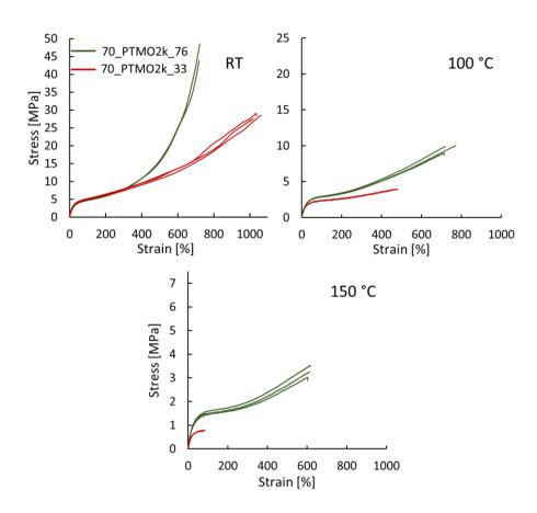
**Figure S3:** Engineering stress-strain curve performed, from left to right, at RT, 100 °C, and 150 °C, at  $\dot{\epsilon}$  = 0.17 s<sup>-1</sup>.
