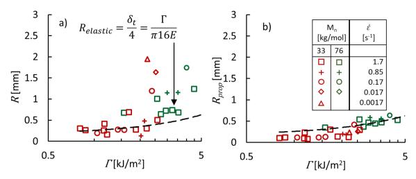
**Figure S4:** Radius of the crack tip right before crack propagation, R, (a) and during propagation,  $R_{prop}$  (b) calculated via parabolic fit of the crack tip.
