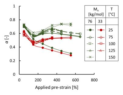
**Figure 2:** a) Relative elasticity,  $\alpha$ , versus applied pre-strain from cyclic tensile tests at different T's for low and high Mw sample. Data points where SIC of the SB is expected to occur are denoted with filled symbols. The data point of Mn=33 kg/mol at T=150 °C is missing because the material fails before being able to complete a full stress-strain cycle.
