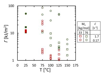
**Figure 5:** Fracture toughness,  $\Gamma$ , versus temperature for different Mw and strain rates noted in the legend. Values for  $\Gamma$  at the other testing conditions are given in Table S1. Data points where SIC of the SB is expected to occur are denoted with filled symbols.
