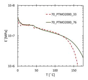
**Figure S5:** Storage modulus of the samples 70\_PTMO2k\_33 and 70\_PTMO2k\_76. Rectangular shaped samples (40 mm long, 2 mm wide) punched out from the 200  $\mu$ m hot-pressed films are tested in tension at heating rates of 5 °C/min and at a constant frequency of 1 Hz. The elastic modulus is measured from DMTA rather than being calculated from tensile tests for convenience and increased accuracy.
