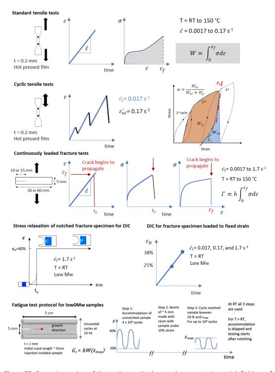
**Figure S2:** General overview of the testing methods, samples geometries and definitions of the variables.
