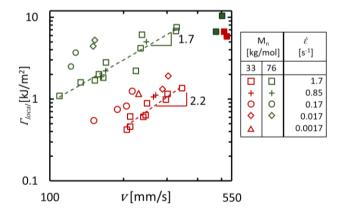
**Figure 8:** Critical energy for crack propagation,  $\Gamma_{local}$ , versus the crack propagation speed,  $\nu$ , at different testing conditions. The fitting with a power law is done only on the data at  $\dot{\epsilon}$ = 1.7 s<sup>-1</sup> (squares) and T > RT. See table S1 for a summary of testing conditions. Data points where SIC of the SB is expected to occur are denoted with filled symbols.
