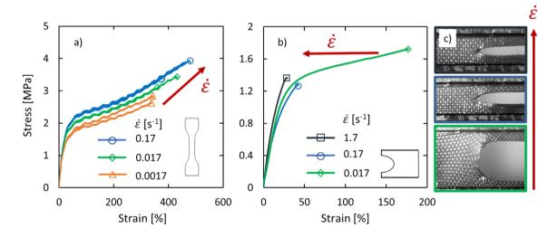
**Figure 6:** Engineering stress-strain curves for a low-Mw sample from tensile (a) and fracture (b) tests at 100 °C and varied strain rates. c) Snapshots of the fracture samples right before crack propagation corresponding, from bottom to top, to the tests performed at  $\dot{\epsilon} = 0.017 \, \text{s}^{-1}$ , 0.17 s<sup>-1</sup>, and 1.7 s<sup>-1</sup>.
