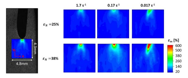
**Figure 9:** The left image shows the  $4.25 \times 4.80 \text{ mm}^2$  area ahead of the crack tip analyzed via DIC. The stretching direction is denoted as x. The local strain fields for low-MW fracture samples tested at RT with nominal strains of 25% and 38% and strain rates between 0.017 s<sup>-1</sup> to 1.7 s<sup>-1</sup> are shown to the right.
