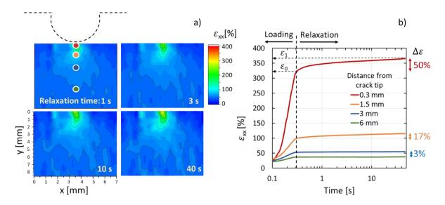
**Figure 10:** a) Local strain field in an 8.5 x 7mm<sup>2</sup> area in front of the crack tip. b) Local strain field versus time at different distances from the crack tip, highlighted in (a) with the same color code. The increase in strain since stress relaxation started,  $\Delta \varepsilon = \varepsilon_1 - \varepsilon_0$ , is noted at the right.
