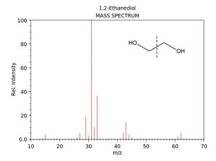
Figure 6. Electron Ionization (EI) mass spectrum of 1,2-ethanediol or ethylene glycol ( $C_2H_5O_2$ ). The base peak is at m/z 31 and is significantly stronger than any other m/z as it represents the perfectly symmetric breaking of the molecule (shown on the top right corner), leaving 2 hydroxymethyl radicals of which either one can keep the positive charge induced by the electron impact. From NIST Chemistry WebBook (https://webbook.nist.gov/chemistry).
