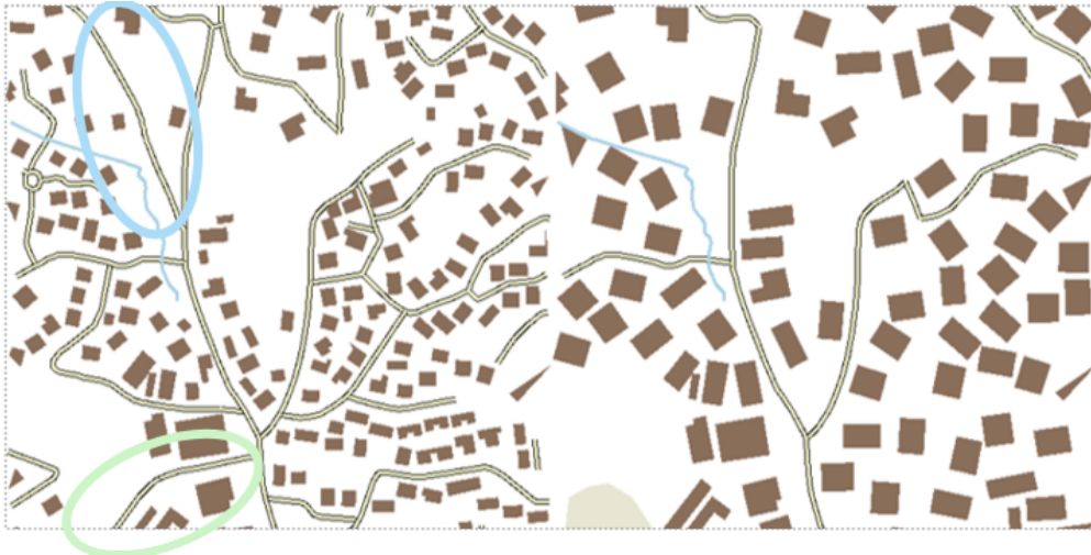
Figure 1: The necessary information to learn the selection of road is not visible in tiled images. The section circled in green is selected because it is a dead-end but the tiling hides this context. The section circled in blue is selected because it is a local path but this information is not symbolised in the tile.
