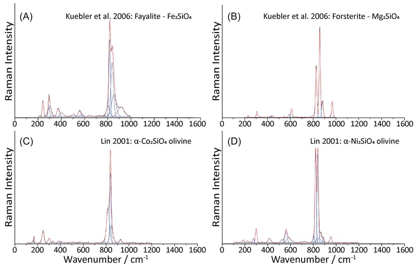
FIGURE 1 Selection of representative spectra from literature (A and B from Kuebler et al.<sup>30</sup> C and D from Lin<sup>31</sup>), corresponding to different olivine compositions, featuring a main Raman peak at  $\sim 820 \text{ cm}^{-1}$ .
