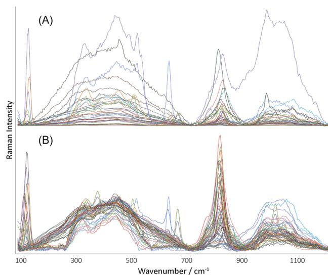
**FIGURE 3** Raman spectra of the studied objects ( $n = 52$ ): (A) after baseline subtraction; (B) then after singular normal variate (SNV) transformation.
