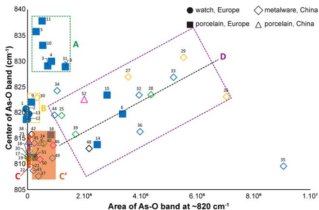
**FIGURE 5** Distribution of the values of the Raman wavenumber of the peak of the main As-O band versus the total area of the band at approximately  $820\text{ cm}^{-1}$ . The numbers indicated correspond to the labels of Table S1.
