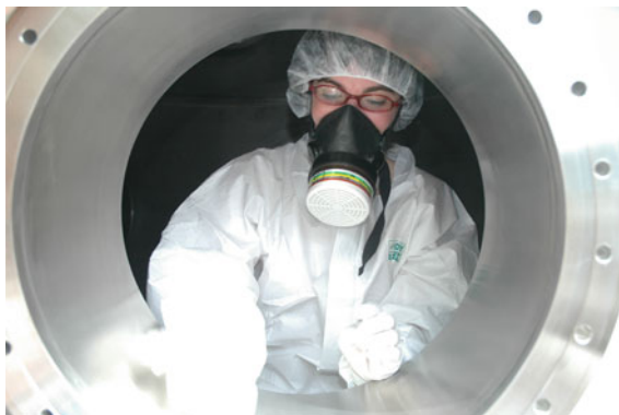
Fig. 3.3 Manual cleaning of an indoor evacuable stainless steel chamber. © LISA-CNRS
