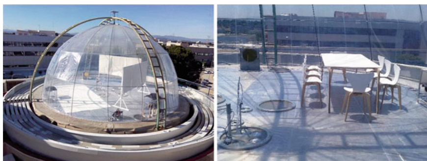
Fig. 7.13 Photocatalytic materials in the EUPHORE chamber. Left: textiles on structures and on the ground. Right: outdoor furniture
