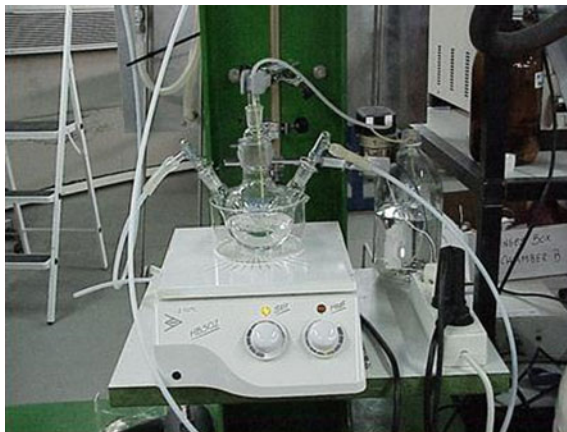
Fig. 4.3 HONO generation system at EUPHORE
