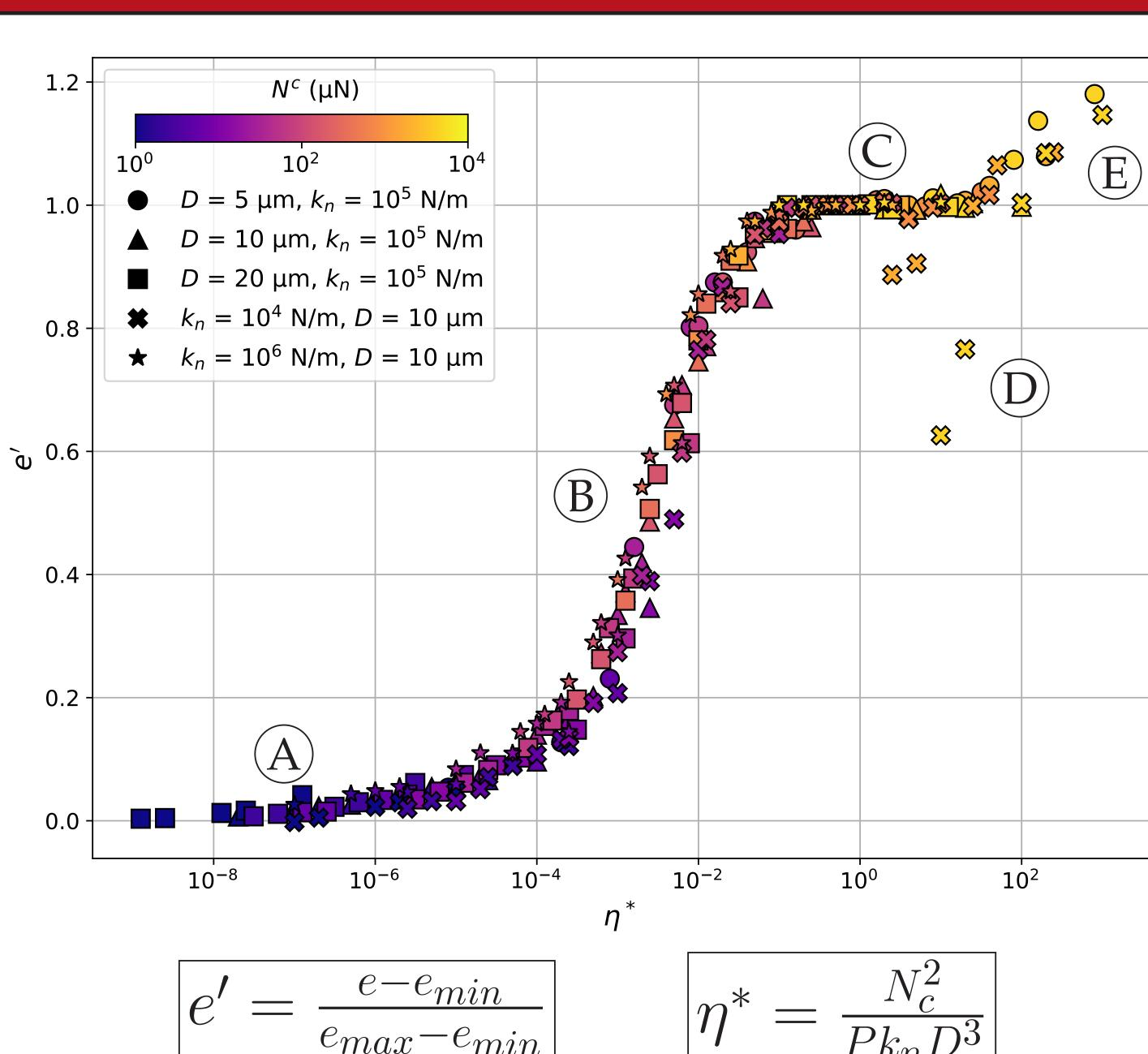
Relative void ratio e' as a function of the dimensionless number  $\eta^*$ , depending on all material parameters and applied pressure. All data points collapse on the same curve except a few points (D & E) that represent special particle configurations induced by rigid walls (see below).
