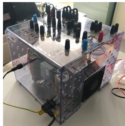
Figure 3 :SEMITEACH Thyristor Power Electronics Teaching System [4].
