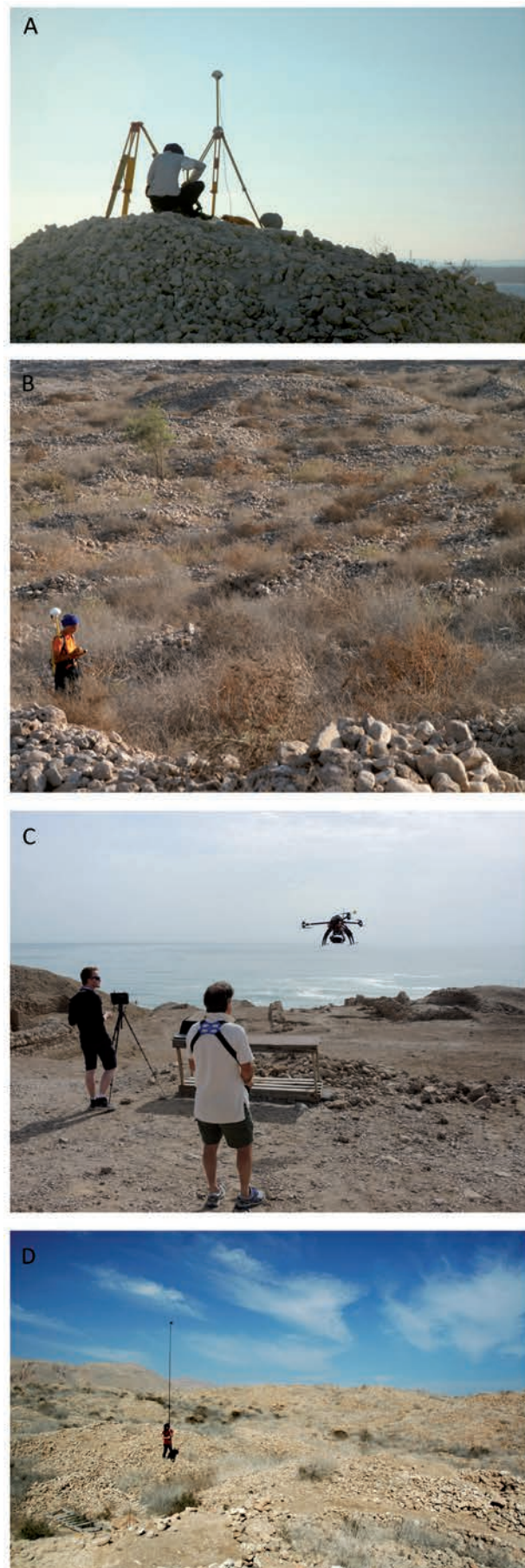
Figure 1.4. The Cartographic Project: A-B) Differential GPS survey (CNRS-Archéorient); C-D) Drone and pole photogrammetry (Iconem).
