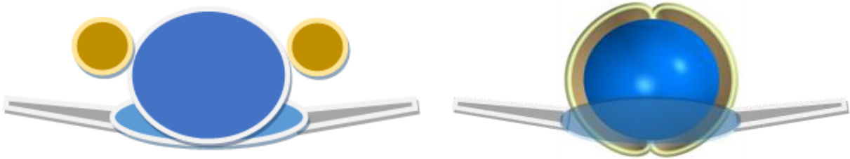
Figure 2 - Comparing a conventional engine installation with the NICE Common Inlet concept.
