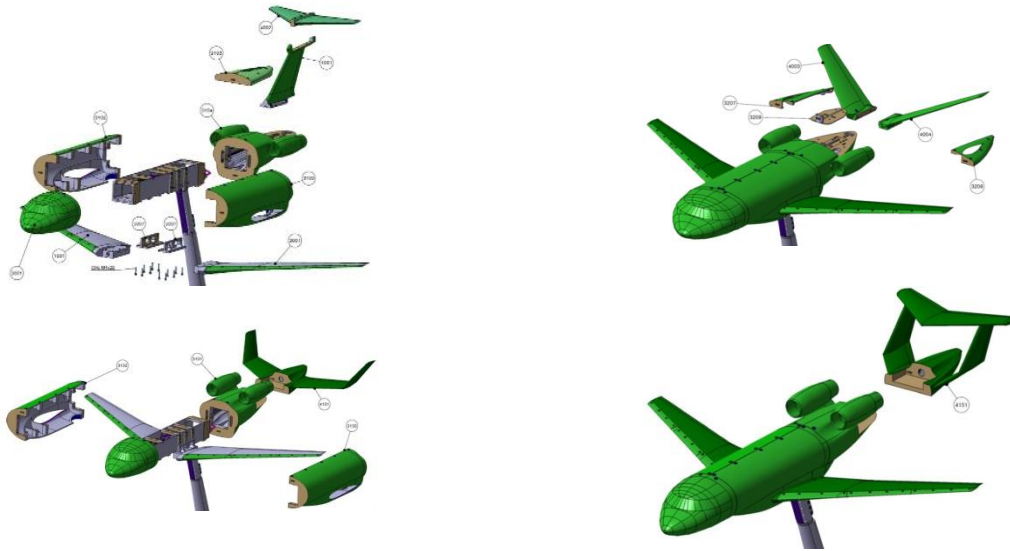
Figure 3 - Modifications of the model to switch from one configuration to the others, illustrated for LF 3.50 m
