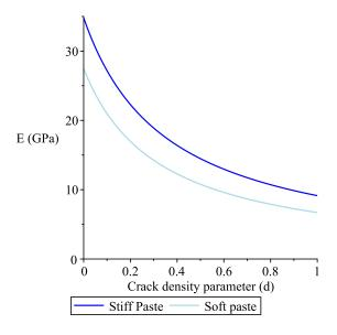
Figure 4: Young modulus in both mortar groups according to crack density evolution
