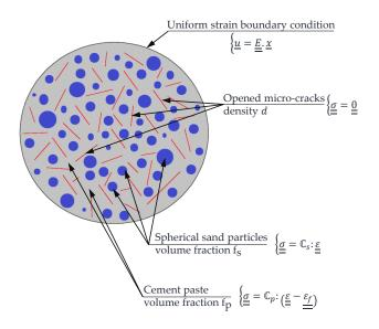
Figure 3: Mortar model with the three phases : cement paste, sand particles and cracks.
