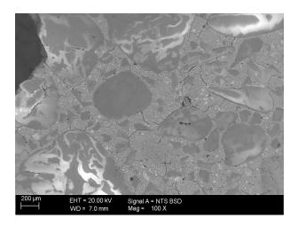
Figure 1: SEM image for 180 days of immersion in water for Normalized CEM I (Y)  $^{\rm tab.1}$  mortar at 0.3% DEF induced expansion.
