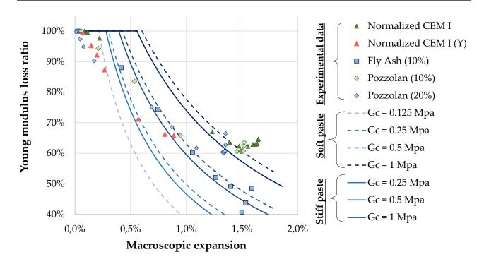
Figure 5: Comparision of experimental results with the model.
