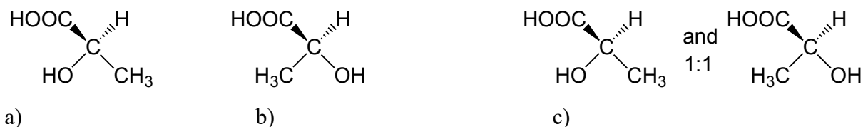
Figure 1. Structures of: (a) ( R )-lactic acid, often termed D-lactic acid; (b) ( S )-lactic acid, widely called L-lactic acid; and (c) a racemic mixture of ( S )-lactic acid and ( R )-lactic acid, called ( RS )-lactic acid or rac -lactic acid.
