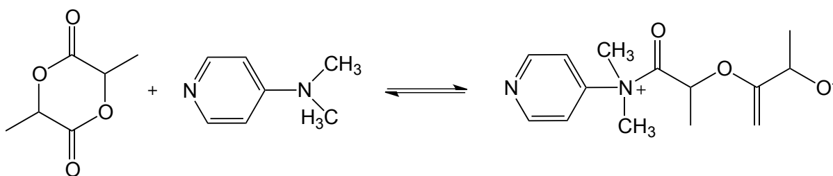
Figure 9. The generation of a zwitterion for the subsequent anionic polymerization of lactides.
