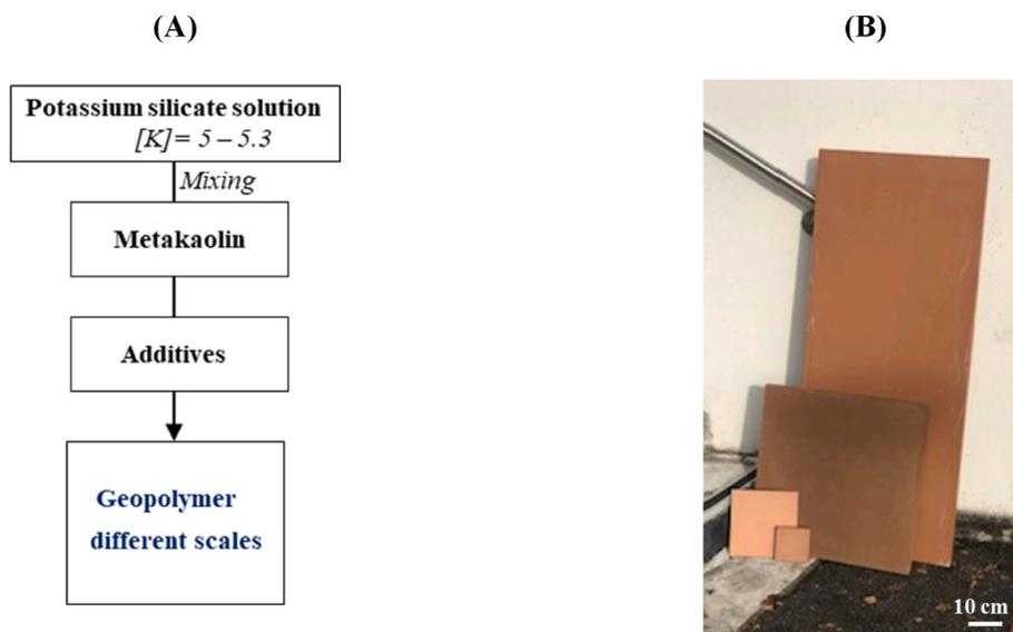
**Fig. 1.** (A) Protocol of the preparation of the geopolymer samples and (B) photo of the geopolymer samples at different scales
