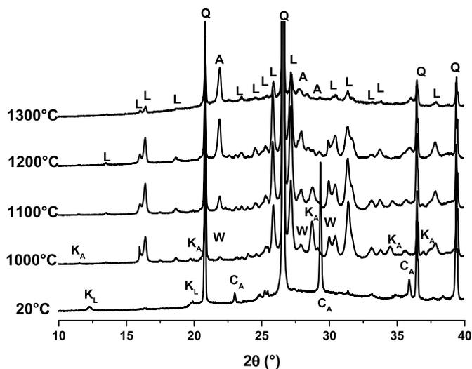
Fig. 4. X-ray pattern of K<sup>6</sup>MS sample treated at different temperature (PDF files: quartz (Q) 01-089-1961, calcite (CA) 00-005-0586, kaolinite (KL) 00-001-0527; kalsilite (KA) 00-002-0297, leucite (L) 01-076-8732, wollastonite (W) 00-002-0629\_00-005-0586 and anorthite (A) 04-011-1371).
