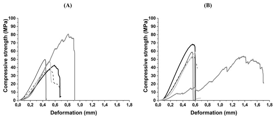
Fig. 3. Evolution of compressive strength as a function of the deformation for (A) K<sup>6</sup>MS and (B) K<sup>5</sup>MS samples treated at (■) 25, (■) 500, (—) 1000, (—) 1100 and (—) 1300 °C.
