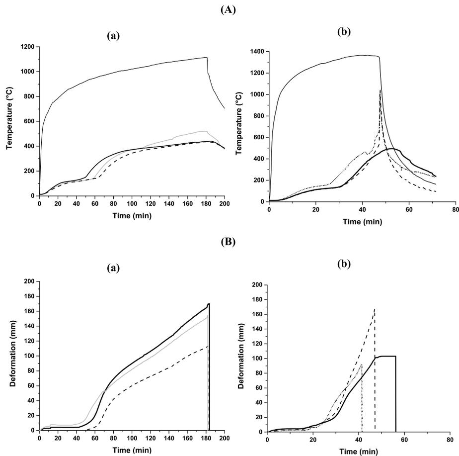
Fig. 9. Evolution of the (A) temperature and (B) deformation as function of the time during the ISO 834-1 standard thermal program (a) and the HCM thermal program (b) for (■, —) K<sup>6</sup>MS, (---) K<sup>6</sup>MSA and (....) K<sup>5</sup>MSA composition.
