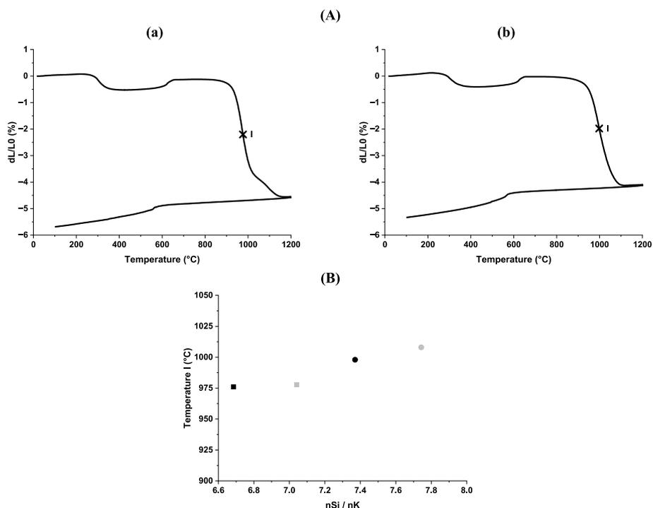
Fig. 6. (A) Dilatometric curves of (a) K<sup>6</sup>MS and (b) K<sup>5</sup>MS samples and (B) evolution of the temperature I according to Si/K molar ratio for (■) K<sup>6</sup>MS, (□) K<sup>6</sup>MSA, (●) K<sup>5</sup>MS, and (○)K<sup>5</sup>MSA samples.
