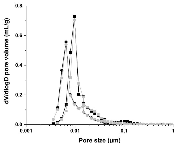
Fig. 2. Values of the (dV/dlogD) pore volume as a function of the pore size for (■) K<sup>6</sup>MS (●) K<sup>5</sup>MS, (▲) K<sup>6</sup>MSA and (●) K<sup>5</sup>MSA samples.
