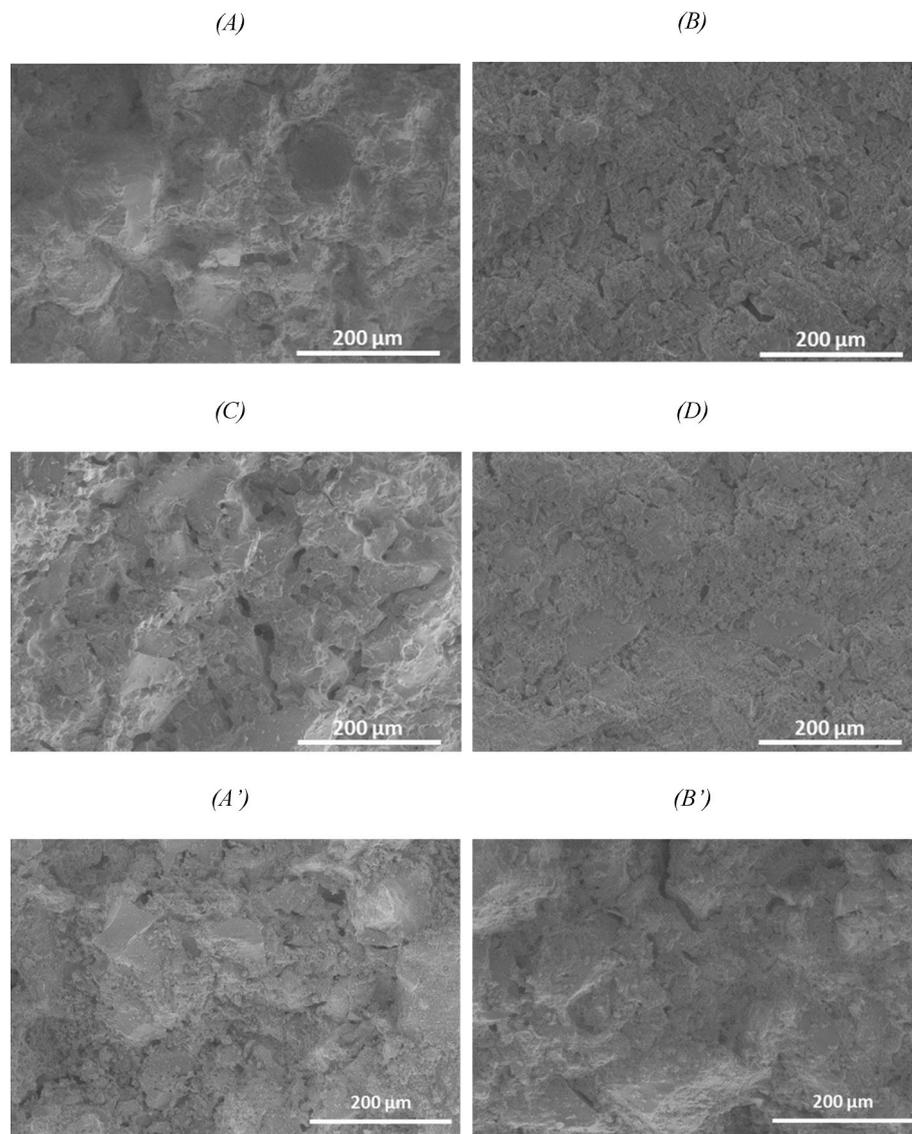
**Fig. 11.** SEM micrographs of (A) K<sup>6</sup>MS, (B) K<sup>6</sup>MSA, (C) K<sup>5</sup>MS and (D) K<sup>5</sup>MSA samples treated at 1000 °C in a laboratory furnace and (A') K<sup>6</sup>MS and (B') K<sup>6</sup>MSA samples treated at Efectis according to ISO 834-1 standard thermal program.
