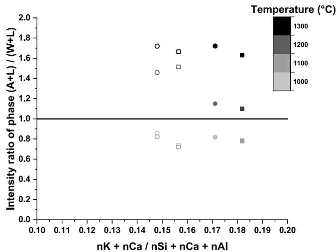
Fig. 5. Evolution of intensity ratio of phase as a function of the K + Ca/Si + Ca + Al molar ratio for (■) K<sup>6</sup>MS, □ K<sup>6</sup>MSA, (●) K<sup>5</sup>MS, and (○)K<sup>5</sup>MSA samples at different temperature.
