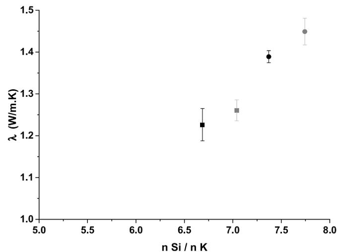
Fig. 10. Thermal conductivity as a function of the Si/K molar ratio for (■) K<sup>6</sup>MS, (○) K<sup>6</sup>MSA, (●) K<sup>5</sup>MS, and (○) K<sup>5</sup>MSA samples.
