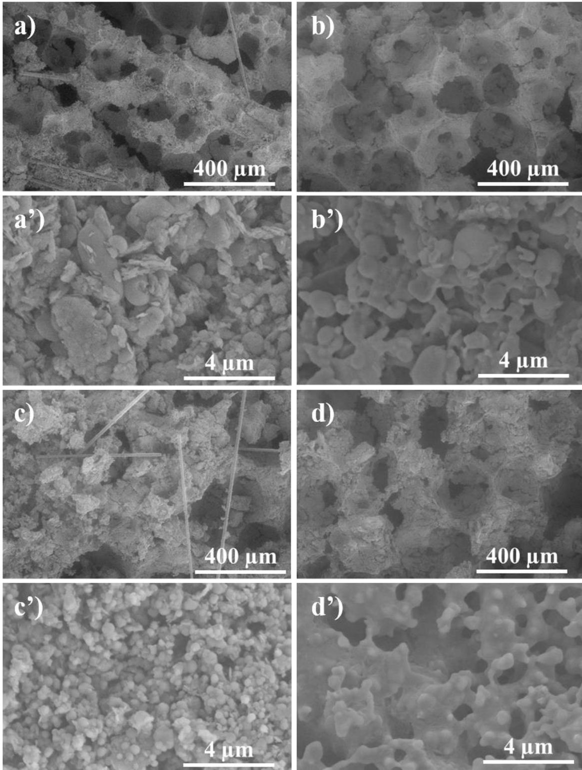
Figure 3: SEM micrographs of (a, a')  $^{2.04}\text{M}_2\text{-F}$  (b, b')  $^{2.04}\text{M}_2\text{-HT}$ , (c, c')  $^{3.10}\text{M}_5\text{-F}$  and (d, d')  $^{3.10}\text{M}_5\text{-HT}$  geopolymer foams at low (a, b, c, d) and high (a', b', c', d') magnification.
