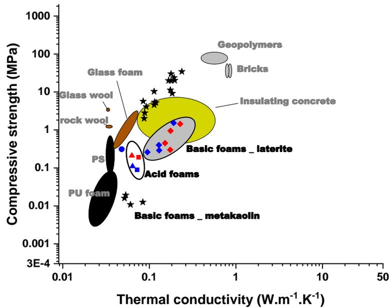
Figure 7: Ashby diagram of ( $\blacktriangle$ )  $^{2.04}M_2$ -based, ( $\blacksquare$ )  $^{3.10}M_5$ -based and ( $\bullet$ ) literature acid-based geopolymer foams samples [27]. Properties of ( $\blacklozenge$ ) laterite [31] and ( $\star$ ) metakaolin [51] alkali-based geopolymer foams. The performances of other insulating materials are also given as a comparison. Note: the blue and red dots indicate room temperature and samples treated at  $1200^\circ\text{C}$ , respectively.
