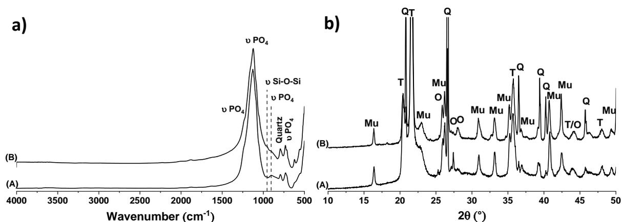
Figure 6: a) FTIR spectra and b) XRD patterns of (A)  $^{2.04}\text{M}_2\text{-HT}$  and (B)  $^{3.10}\text{M}_5\text{-HT}$  geopolymer foams after thermal treatment at  $1200^\circ\text{C}$ . ((Mu) mullite, 01-079-1456, (Q) quartz, 01-070-7344, (O) orthorhombic  $\text{AlPO}_4$ , 04-014-2298 and (T) triclinic  $\text{AlPO}_4$ , 04-012-4467).
