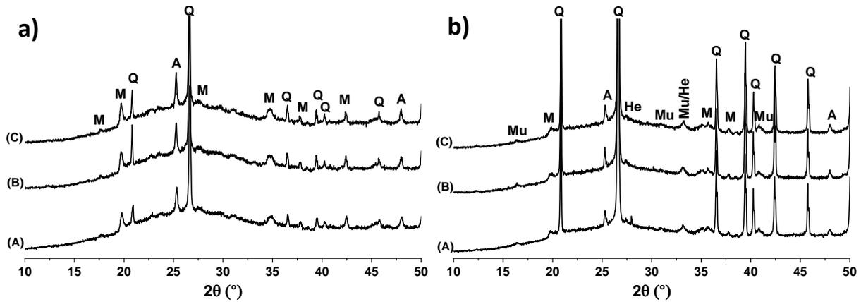
Figure 5: (a) XRD diagrams of (a)  $^{2.04}\text{M}_2$ -based and (b)  $^{3.10}\text{M}_5$ -based geopolymer foams samples under different conditions: (A) fresh, (B) water immersion and (C) freeze-thaw cycle. ((A) anatase, 00-021-1272, (Mu) mullite, 01-079-1456, (M) muscovite, 01-082-3722, (Q) quartz, 01-070-7344, (He) hematite, 01-079-1741)
