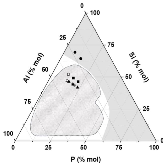
Figure 1: ternary diagram showing the synthesized geopolymer foams, using ▲ M<sub>2</sub> (Δ2.04), ■ M<sub>5</sub> (□ 3.10), ● A<sub>600</sub>, ◆ A<sub>700</sub> and ◇ laterite. In addition, the hatched (▨) and shaded (▩) zones show the feasibility and non-consolidation zones determined for dense samples [36].
