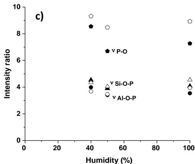
Figure 4: (a) FTIR of (a)  $^{2.04}M_2$ -based and (b)  $^{3.10}M_5$ -based geopolymer foams samples under different conditions: (A) fresh, (B) water immersion and (C) freeze-thaw cycle. (c) Relative evolution of the intensities from the different identified contributions as a function of humidity for geopolymer samples (full)  $^{2.04}M_2$ -based and (empty)  $^{3.10}M_5$ -based samples. (▲,△) formation of an Al-O-P network, (▲,△) Si-based network and (●,○) P-based network.
