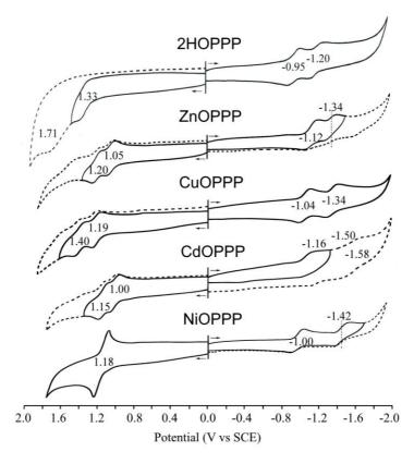
**Figure 2.** Cyclic voltammograms of porphyrins of **OPPP** series in CH<sub>2</sub>Cl<sub>2</sub> containing 0.1 M TBAP.
