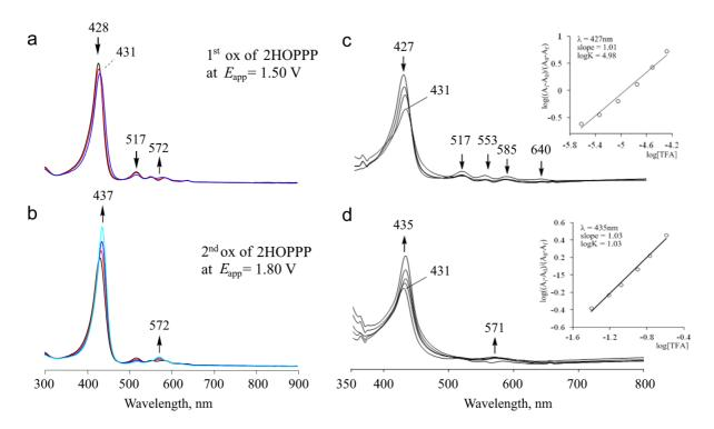
**Figure 3.** Spectrophotometric changes during controlled potential oxidation of **2HOPPP** in  $CH_2Cl_2$  containing 0.1 M TBAP at (a)  $E_{app} = 1.50$  V and (b) at  $E_{app} = 1.80$  V with comparison to spectral changes during acid titration of **2HOPPP** with TFA (c, d). Insets show the treatment of titration data by using Hill plot method.
