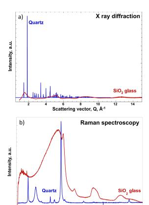
**Figure 3.** (a) X-ray diffraction, (b) Raman spectrometry in blue (quartz or low-cristobalite) and  $SiO_2$  amorphous in red. For practical reasons, spectra are reported in arbitrary units. The conditions of acquisition of the spectra of the crystalline and amorphous phases are different for the same technique and from one technique to another [redrafted from Cormier and Neuville, 2022].
