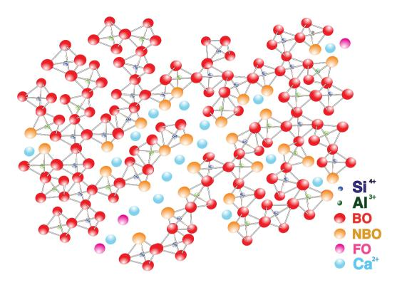
**Figure 5.** Structural sketch of a calcium alumino-silicate glass.
