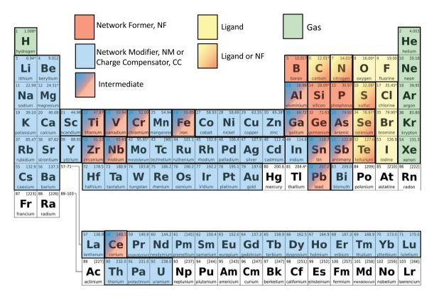
**Figure 1.** Periodic table with possible role of elements in glass or melt. Elements in white can be in glass without any specific role. Elements in white are almost never investigated in glass structure, but they can be present in a glass probably as a gas or network modifier.
