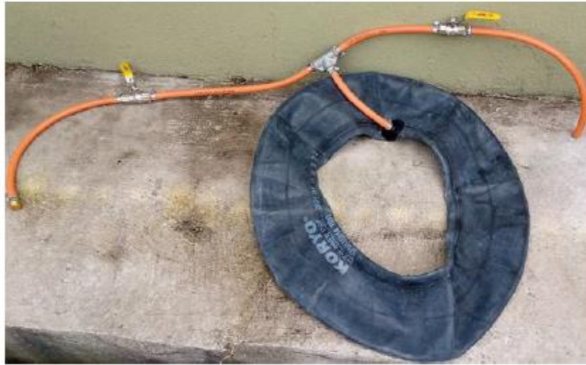
Fig 6: Raw gas storage tank assembly
