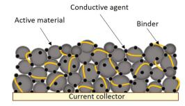
Fig. 7. Schematic representation of a typical electrode structure.
