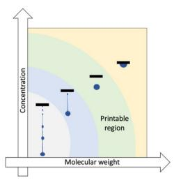
Fig. 8. Four regimes in inkjet drop generation as a function of concentration and molecular weight of polymer.
