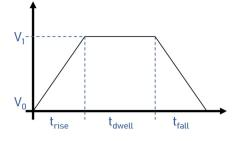
**Fig. 6.** Typical trapezoidal voltage waveform applied to the piezoelectric material in DOD inkjet printing.
