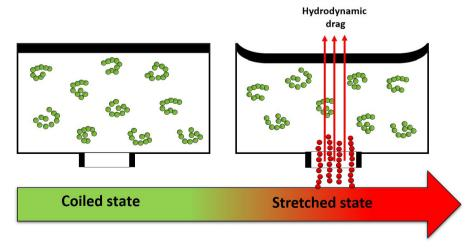
Fig. 9. Schematic representation of strain hardening phenomenon: a) coiled state of polymeric chains, when no stress is applied b) stretched state of polymeric chains during the ejection.
