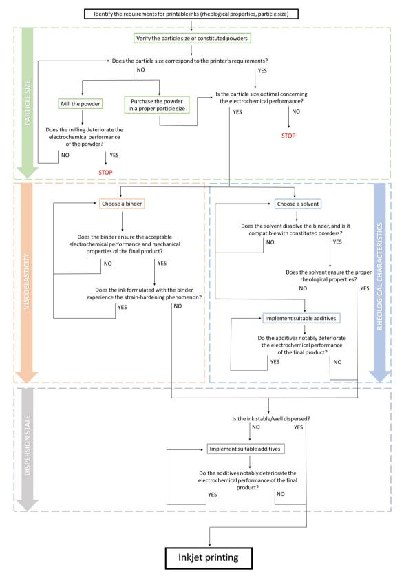
Fig. 2. Detailed flowchart of the fabrication process of electrodes ink.
