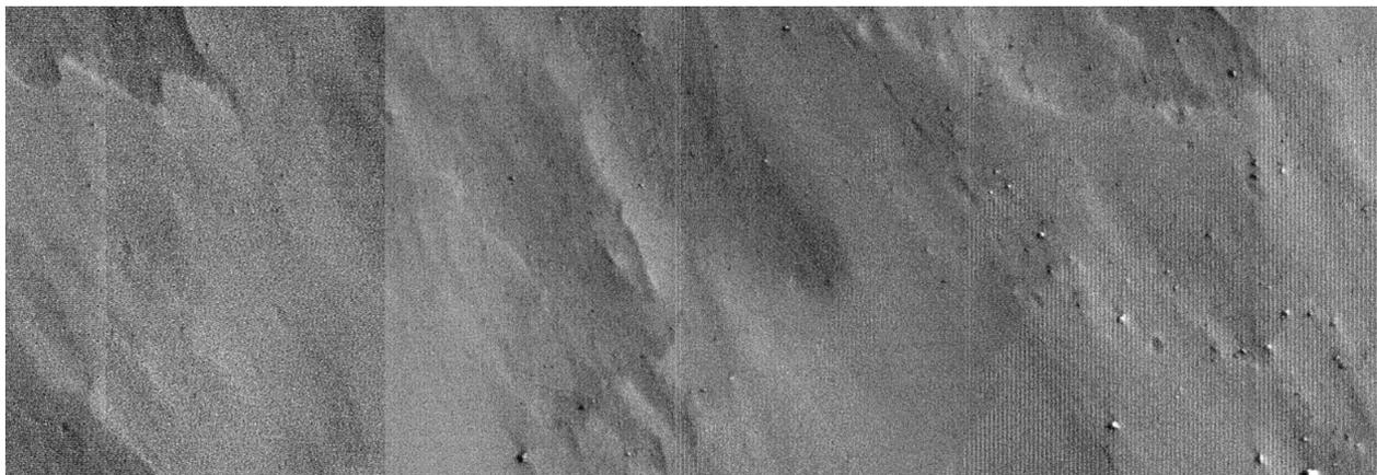
Fig. 19. Bland portion of RED3\_1 of ESP\_074443\_1790 showing minor noise (mostly vertical pattern) due to minor bit-flips. Raw image geometry with north down, image width 0.5 km.
